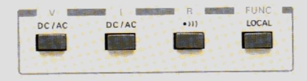
Current, voltage and resistance measuring can be selected directly using the corresponding function keys. After the mains voltage has been switched on,
